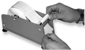
Feed liner between second bar and coiled third bar.
